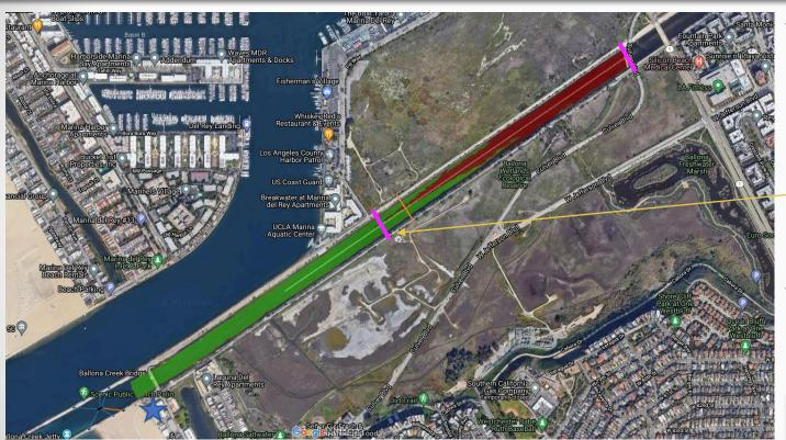
The magenta line indicates the most upstream the Interceptor could feasibly be placed downstream based on creek elevations
